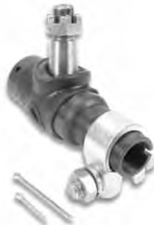
STEER CYLINDER ROD END Stud Thread ..... 3/4-16 Shaft Thread ..... 1-1/16-12 Internal
