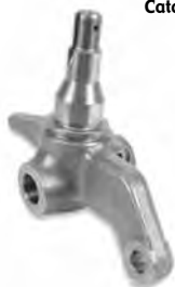
KNUCKLE RH-TOYOTA Thread ..... M24 x 1.5mm
