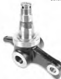
KNUCKLE RH-KOMATSU Thread ..... M30 x 1.5mm
