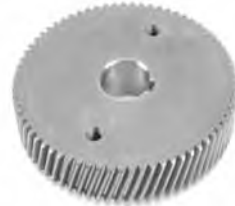
STEER GEAR O.D. .... 4.590" # of Teeth ..... 69
